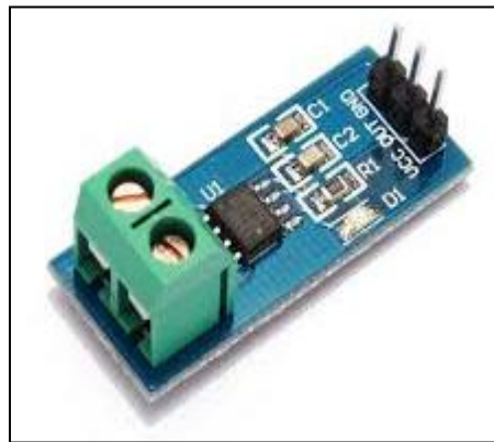
Figure 4: ACS712 Current Sensor
